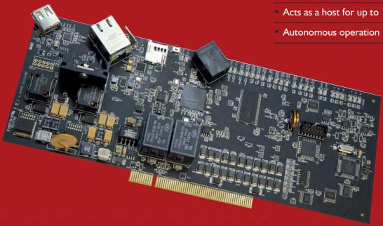
The entronet controller is an intelligent field device which incorporates an independent two door controller capable of making access control decisions without reference to entrowatch.
