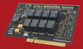
The IOM is a compact general purpose I/O module which can be integrated with external devices such as fire alarms, heating & lighting panels etc.
