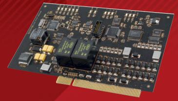
The entronet TDEM is a two-door access control module which can be plugged into an entronet backplane.
