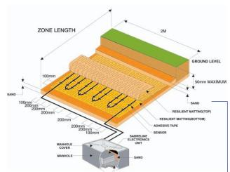
SabreLine sensor cable provides the ideal solution for buried applications in sterile areas or over open ground where effective detection of intruders is essential.
