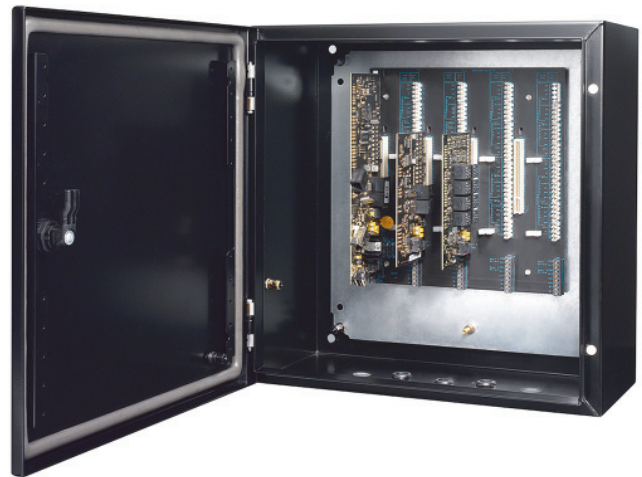
ACP II with optional TDEM and IOM in a 4 way backplane
